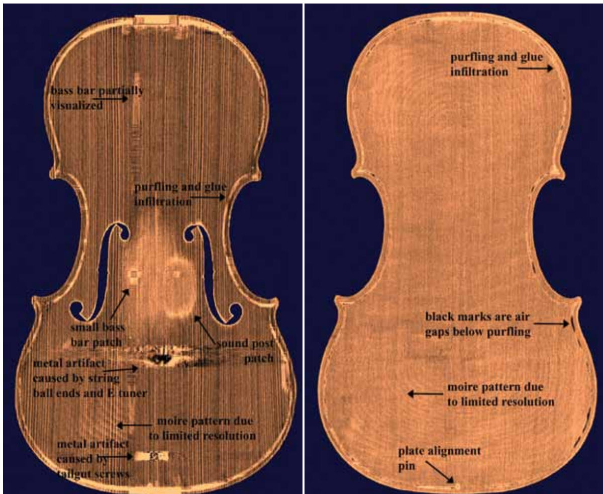
Figure 4. Density maps (generated from the MP) of the top and back of a violin by Guarneri del Gesù dated 1735.
