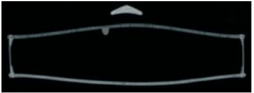
Figure 2 transverse CT profile of a 1735 Guarneri 'del Gesù' at the widest section of the lower bout. Note end of bass-bar (within body) and part of tailpiece (above body)
