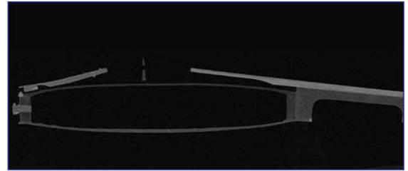
**Top:** This CT image shows a “sagittal” view of a rare violin. **Left:** This transparent view of a violin box came from adjusting volume rendering parameters, allowing for an “inside” look at the violin’s sound post and bass bar.
