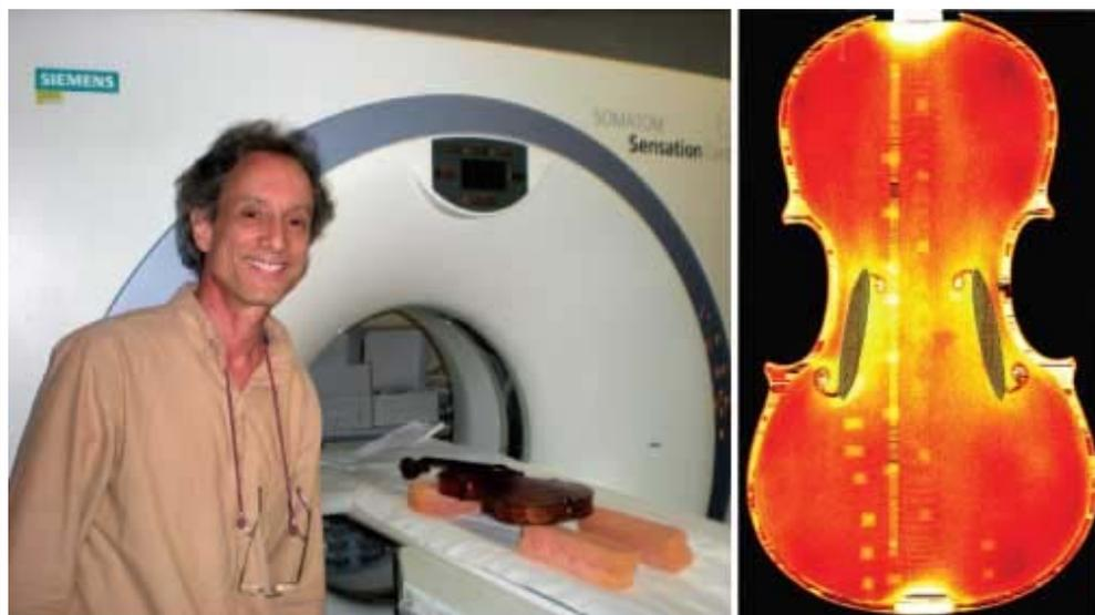
Terry Borman and the CT machine, left, and a scan of a violin, showing many crack-stabilizing cleats.
